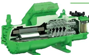
All ElectraTherm ORC systems are powered by BITZER's semi hermetic, twin screw expander. This allows ElectraTherm's ORC process to utilize much more variable heat sources than leading turbine technologies thanks to greater transient operation that allows for "wet" dual-phase flow and greater turndown ratios allowing for continuous power generation when dealing with inconsistent thermal input.
